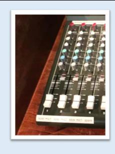
N.B. The HAND HELD MICROPHONE when used in a stand may require a slightly higher setting on the slider, than the LAPELS.
