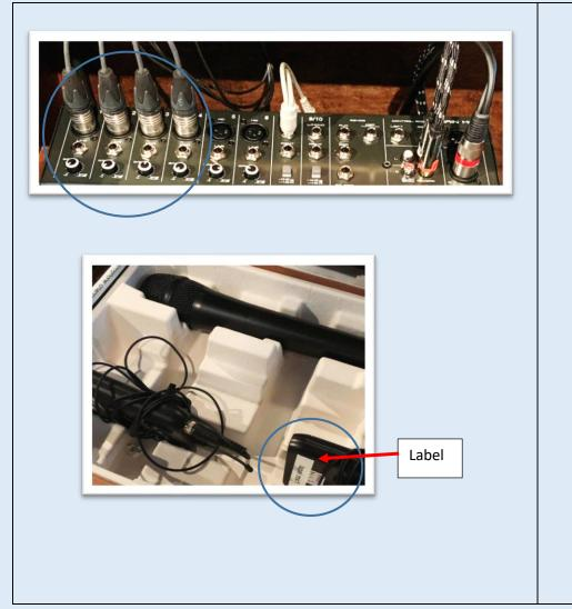
2. The inputs for the Microphones are all pre-wired back to the microphone receivers so there is nothing to plug in!
